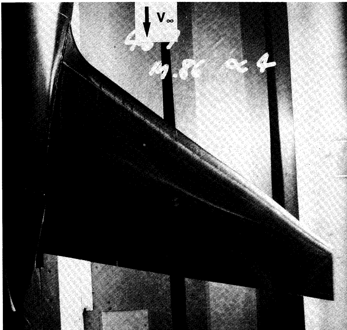
Fig. 4 Horizontal tail in the Boeing Transonic Wind Tunnel.
