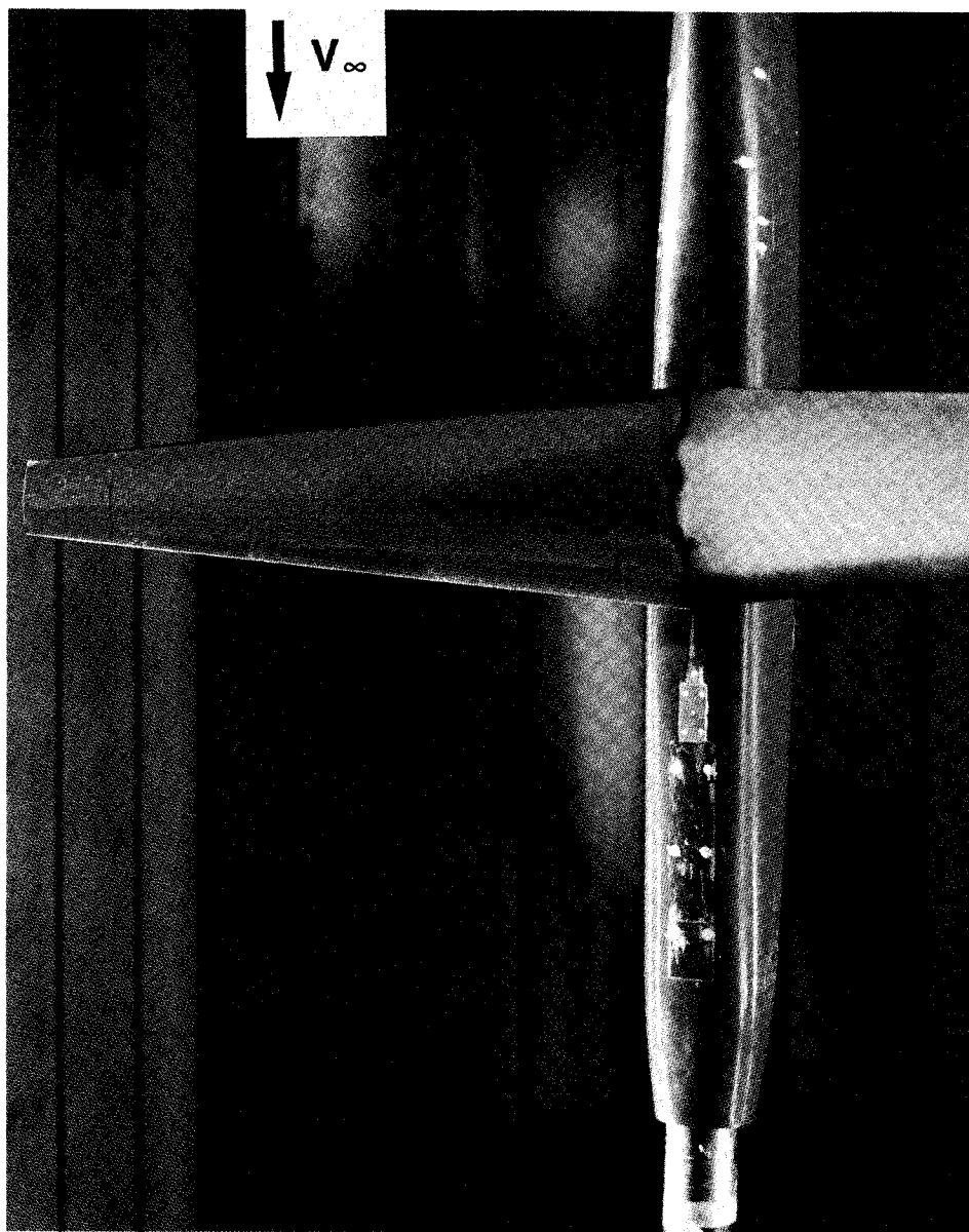
Fig. 5 Unswept supercritical wing in the NASA Ames 11-ft Transonic Wind Tunnel (sublimation on right side, liquid crystals on left side).
